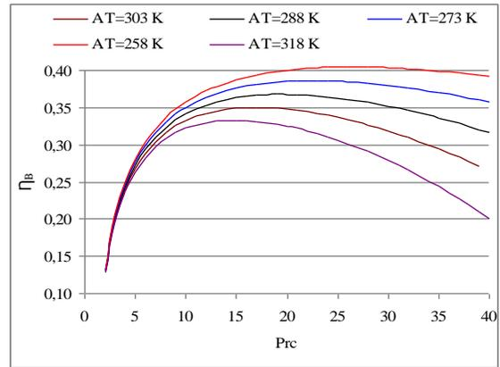
**Fig. 2. The Variation of the Total Efficiency ( $\eta_B$ ) Of Simple Brayton Cycle with Compressor Pressure Ratio ( $P_{rc}$ )**
