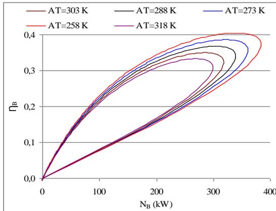
Fig. 4. The Variation of the Total Efficiency ( $\eta_B$ ) with the Net Power ( $N_B$ ) of Simple Brayton Cycle
