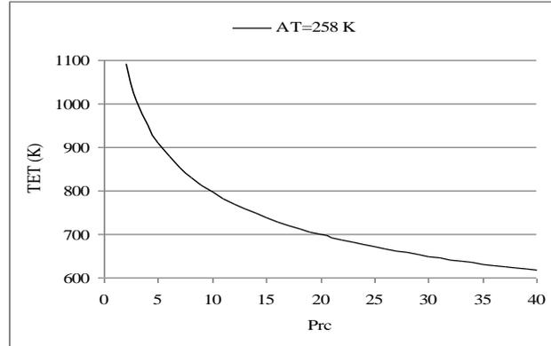
Fig. 5. The Variation of the Turbine Exit Temperature (TET) With The Compressor Pressure Ratio of Simple Brayton Cycle
