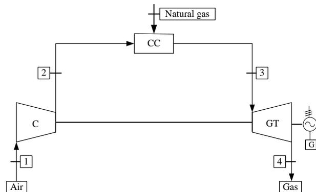
Fig. 1. The Flowchart of Simple Brayton Cycle
