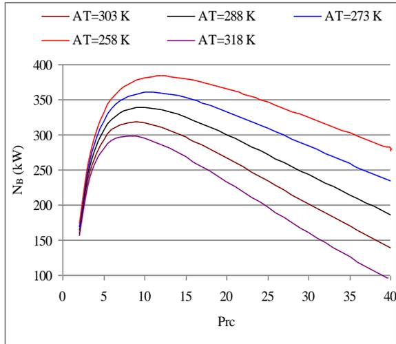
Fig. 3. The Variation of the Net Power ( $N_B$ ) of Simple Brayton Cycle with Compressor Pressure Ratio ( $P_{rc}$ )
