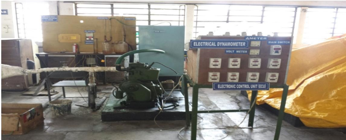
Figure 1: Kirloskar Single Cylinder Four Stroke Air Cooled C.I. Engine with Electrical Dynamometer
