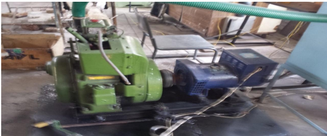
Figure 2. Engine coupled with electrical dynamometer
