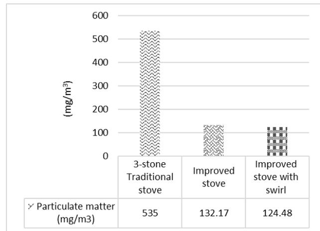
Fig. 9 Particulate matter test results
