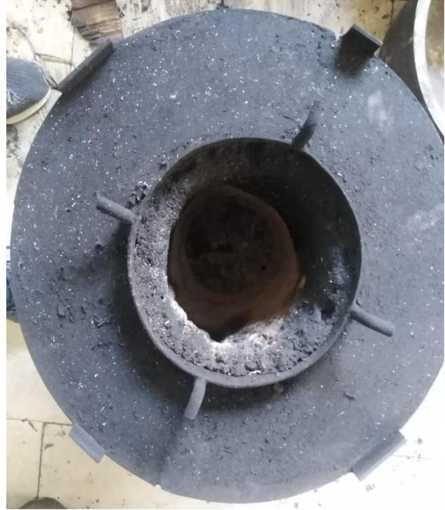
Fig. 2 Top view of test improved cookstove
