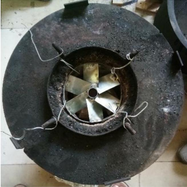
**Fig. 4 Swirl set up on top of the improved cookstove.**
