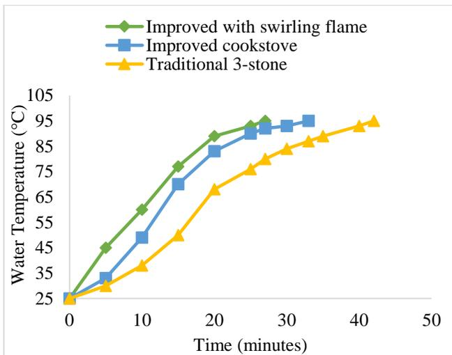
Fig. 6 Variation of the temperature of the water with time in all three cookstoves
