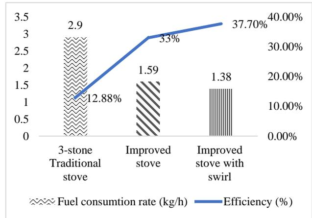
Fig. 8 Efficiency and fuel consumption in stoves
