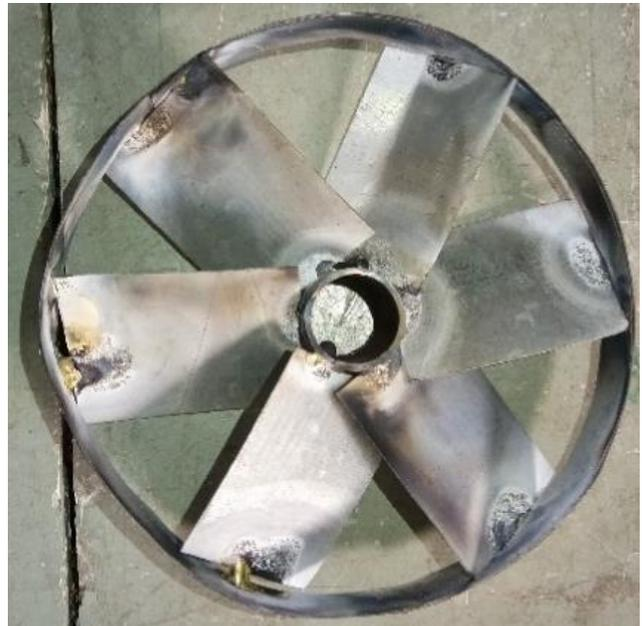
Fig. 3 Swirl 6-vane burner
