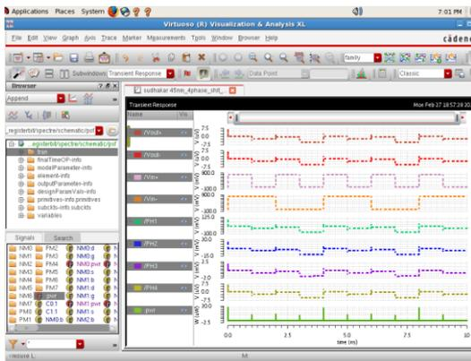
Figure 14 4-Phase Shift Register Bit Of Output Waveform
