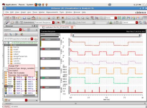
Figure 10 Basic 2N-2N2P Buffer/Inverter Output Wave form at Frequency 100mhz.
