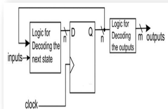
Fig 5. Finite State block diagram
