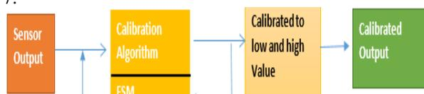
Fig.7 . Diagram represents algorithm used in two point technique
