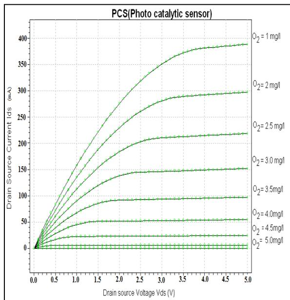
Fig. 4. characteristics curves for different value of oxygen content
