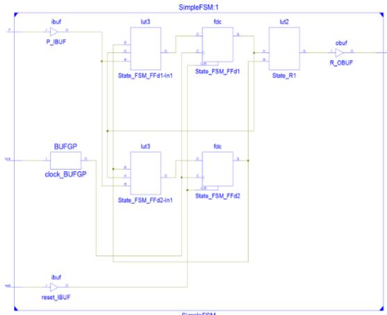
Fig. 6 .RTL of finite state Machine
