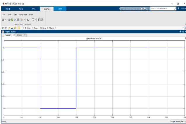
Figure 6: Gate pulse of the power electronic device used
