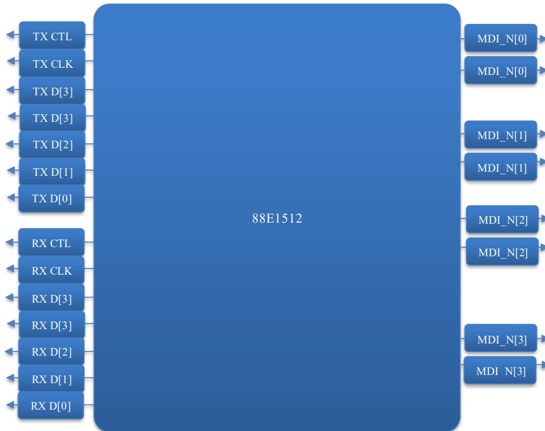
Fig. 9 Block Diagram of Ethernet Interface
