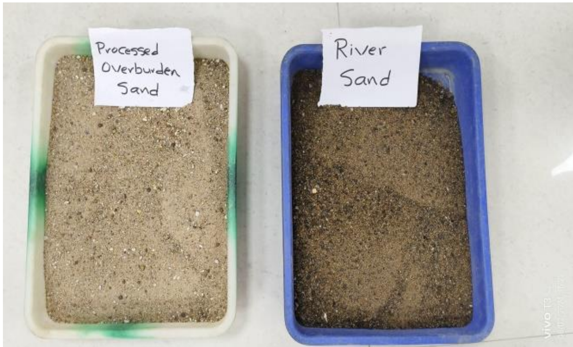
Fig. 1 Processed Overburden Sand (OBS) and Natural River Sand (RS) fine aggregates
