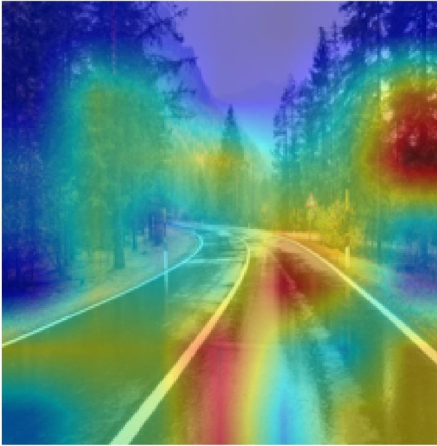
Fig. 9 Grad-CAM visualization highlighting the areas of focus in the road surface during classification
