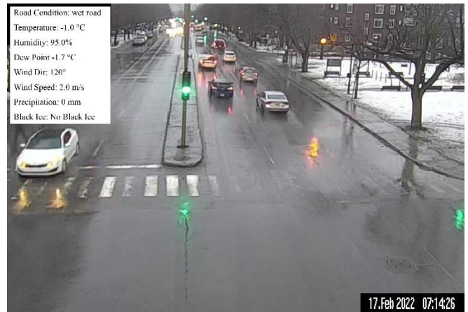
Fig. 13 Wet road scenario with sensor data
