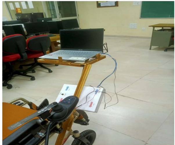
Fig. 4 Physical model developed for real-time control of an Electric wheelchair
