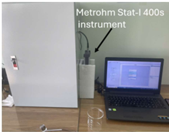
Fig. 2 Electrochemical corrosion measurement, (a) Electrochemical corrosion test setup, and (b) Electrochemical corrosion measurement process.
