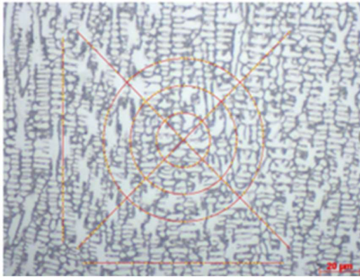
(b) Fig. 4 Grain size of the sample at the coating region, (a) Original image, and (b) Image with annotations.
