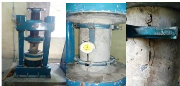
Fig.5: Modulus of Elasticity Test Setup
