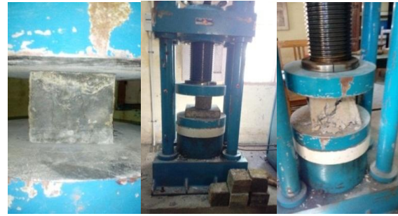
Fig.2: Compressive Strength Test Setup
