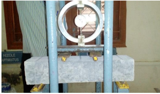
Fig.4: Flexural Strength Test Setup.
