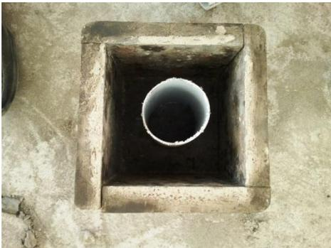
Fig2 (b) 4.5cm pipes in concrete cube
