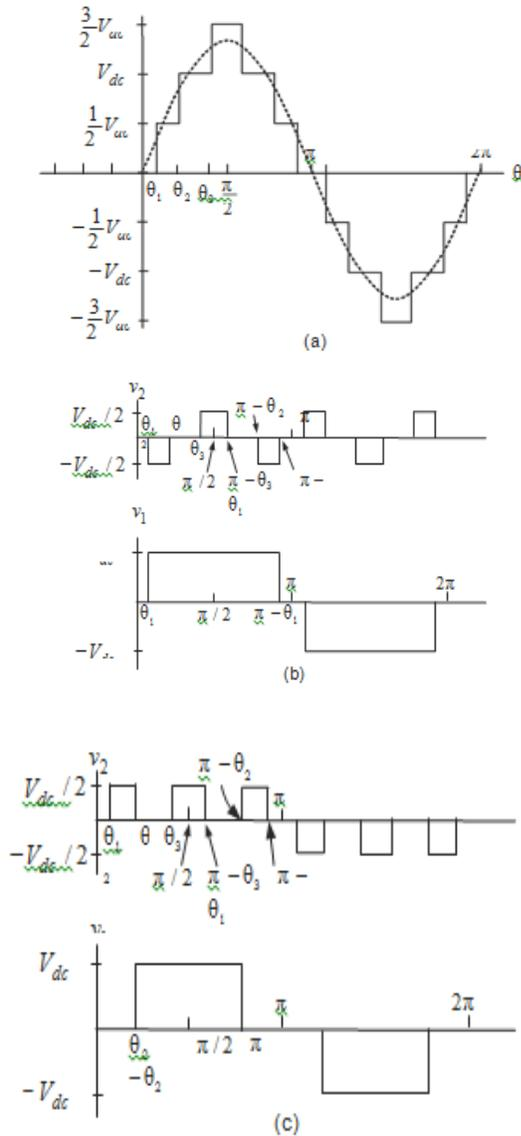
Fig. 2. (a) Output waveform of an 7-level cascade multilevel inverter. (b) and (c) H-bridge voltages  $v_1$  and  $v_2$  which achieve the same output voltage waveform  $v = v_1 + v_2$ .
