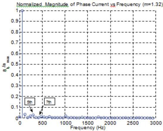
Fig. 6. FFT of the phase current for  $m = 1.32$  and  $f = 60$  Hz.
