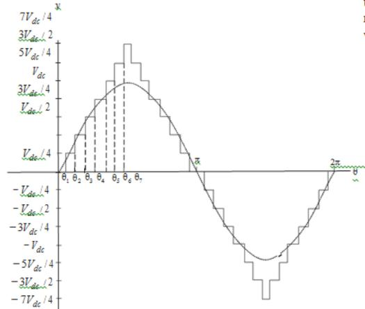
Fig. 8. Hardware architecture and output voltage waveform for a 15-level inverter.
