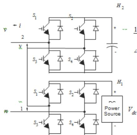
Fig. No. 1. Single-phase structure of a multilevel cascaded H-bridges inverter.
