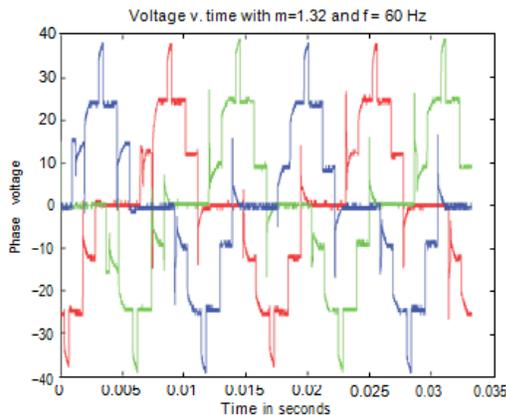
Fig. 3. Three-phase output waveforms of the seven-level multilevel inverter. Note that the second level in Fig. 3 is constant at 25 V because this level is due to only the power
