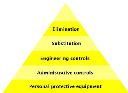
Figure 1.7.1: HIERARCHY OF CONTROLS
