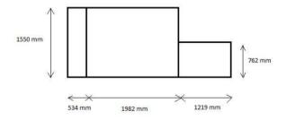
For the volume calculation, the shape of the car is considered into rectangular segments and the buoyancy calculation is proceeded Where the car's width = 1690mm Volume of 1st segment = 1\*b\*h = 1550\*534\*1690 = 1398813000 sq.mm
