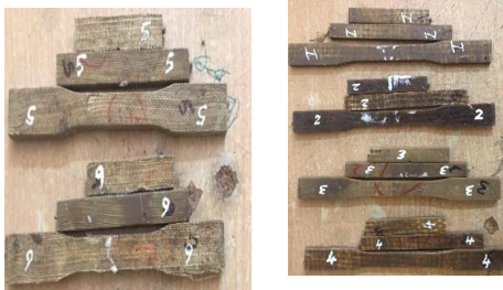
Fig 1: E-GF( 25%)+Resin (75%)+ vajram (85%)+ Epoxy(15%) plate
