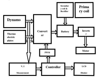
The electric and fuel vehicles system consists of dynamo, thermo electric plate, converter, battery,
