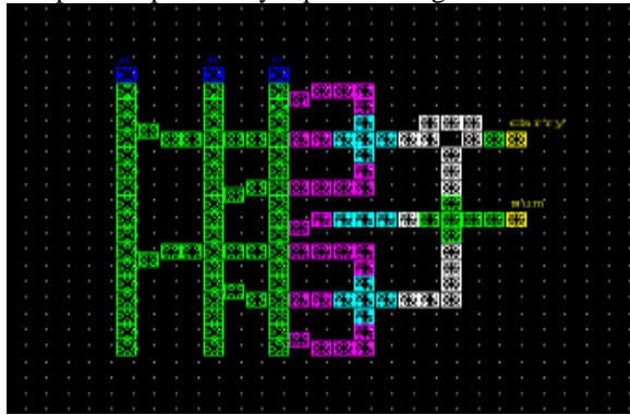
FIGURE :8 QCA Layout Of Conventional one-bit QCA full adder
