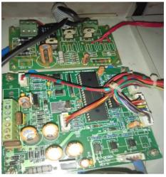
Fig. 3. Power loom Control
