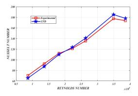
Figure 5.1.2 Comparison of Experimental and numerical results for Twisted square duct. with insert
