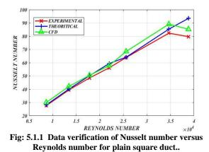
The graph represents variation of Nusselt number with Reynolds number for plain square duct using air is test fluid The experimental values were compare with standard equation. It was observed that Percentage deviation between experimental and theoretical values is
