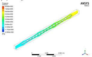
Figure : 5.2.3 pressure contour of Twisted squure duct with circular rod at velocity of 2.2 m/sec
