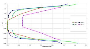
Figure : 5.2.5. Temperature profile of Twisted squure duct with cirular rod at velocity of 4.5 m/sec.
