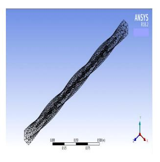
Fig 2 Twsited duct with circular rod insert meshing
