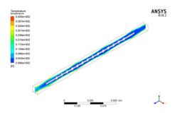
Figure : 5.2.4 Temperature contour of Twisted square duct with cirular rod at velocity of 4.5 m/sec.
