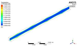
Figure : 5.2.9. Temperature contour of Twisted square duct with cirular rod at velocity of 8.6 m/sec.
