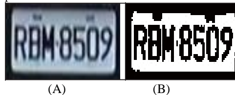
Fig.3. an example of a detected vehicle license plate, (b) a binarized plate
