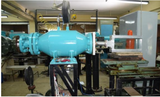
Fig 5: Vacuum Ejector - Diffuser Experimental Set Up
