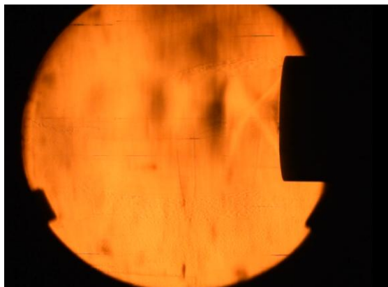
Fig 12: Shock Train Formed inside the Model
