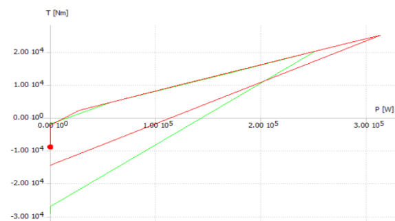
Fig 7: TORQUE VS POWER COMPARISON OF STRAIGHT AND SWEPT BACK TURBINE
