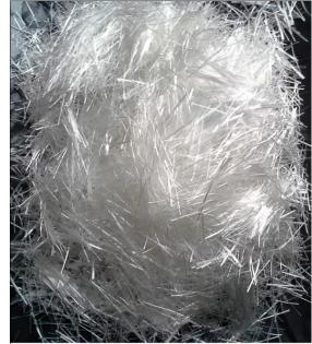
AR GLASS FIBERS Fig1: AR Glass Fibers
