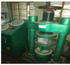
Figure 8.1: Picture showing the compressive testing for cubes
