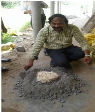
Mixing of concrete with banana fibres
