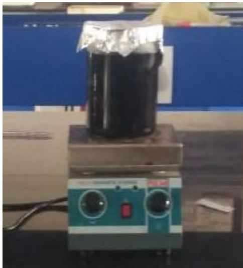
Fig. 1 CNT dispersion in water after sonication
