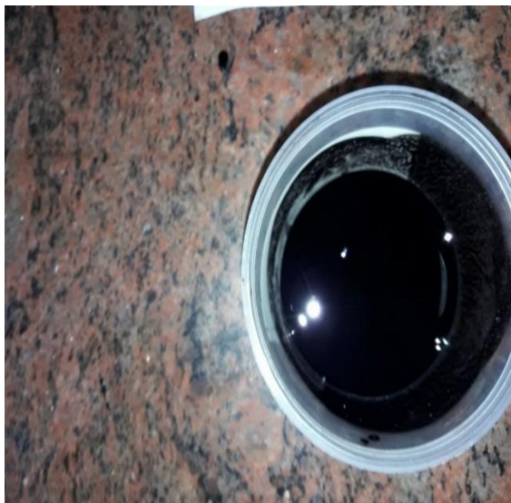
Fig 3.2. Lignin mixed with kerosene
