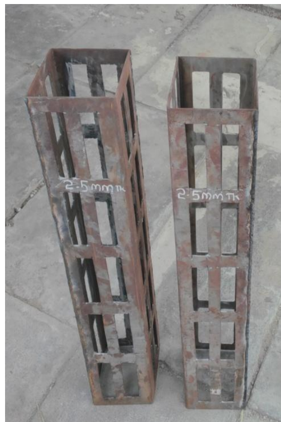
Fig 3. Prefabricated cage system (Double opening)
