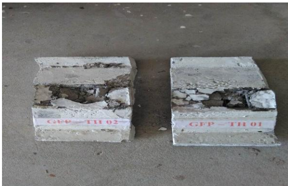
Figure 7. Geopolymer Ferrocement Trough Panels at failure
