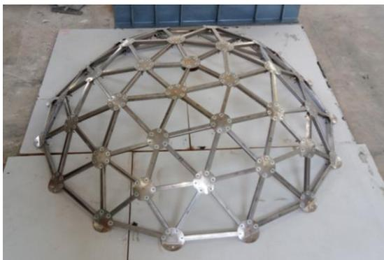
Figure IV. Completed structure of Tessellation dome.
