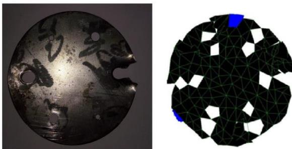
Analytical and Experimental Specimen comparison is not satisfactory, this is because of nodes generated manually and deviations and slip in joints of the plate and bolt, is observed experimentally. Since the plate failed only after peak load of 7kN which is far for the scaled model, the plate of 1mm thickness and bolt of 4mm is adopted.
