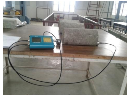
Figure 1 Ultrasonic Pulse Velocity Test
