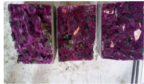
Fig 6. Carbonation test setup
