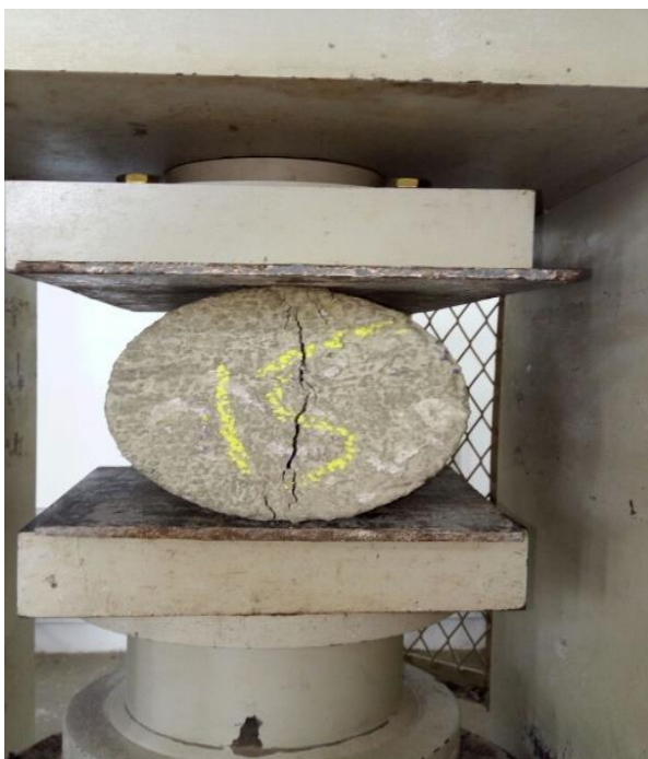
Fig 4.2 Specimen for Split tensile
