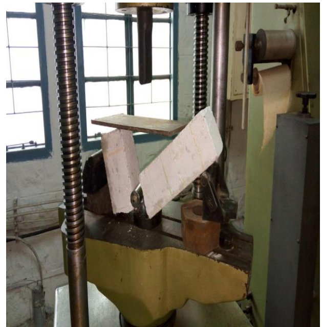
Fig 4.3 Specimen for Flexural test
