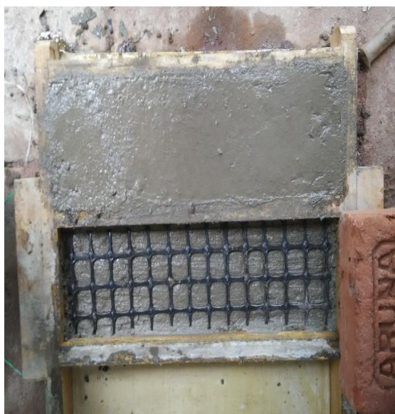
Fig 5: Placing of layers in mortar
