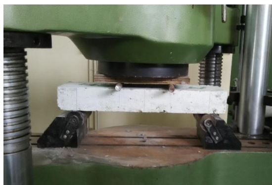
Fig 7: Flexural testing on panels
