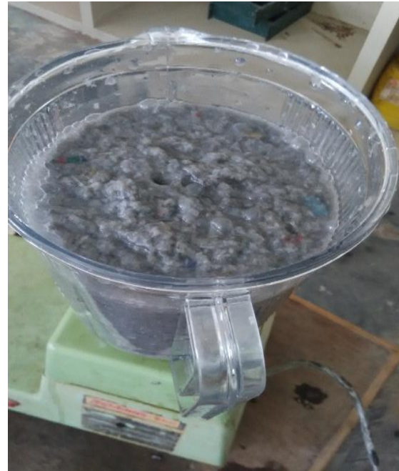
Fig 2: Paper pulp preparation
