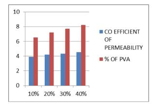
Figure 2: permeability values for varying % of PVA
