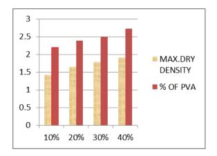
Figure 1: Max. dry density for varying % of PVA
