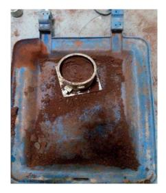
Figure 1.a: Standard proctor compactor
