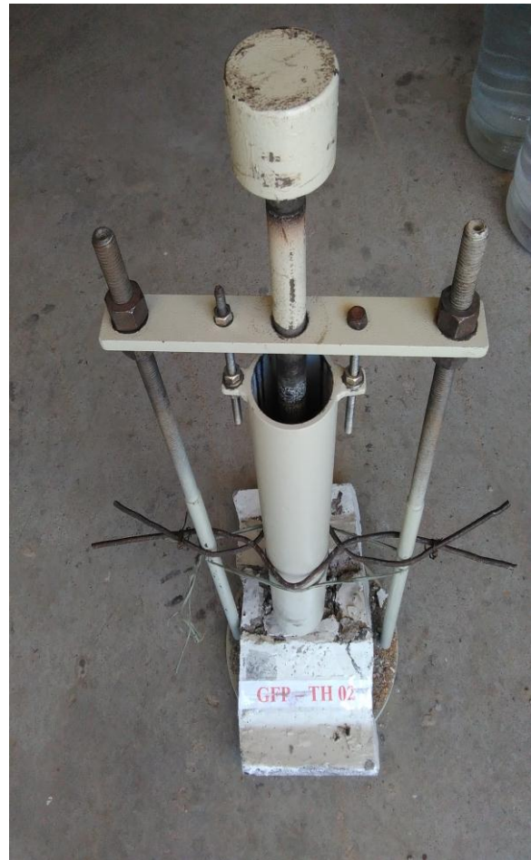
Figure 2. impact machine set-up
