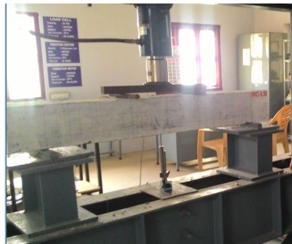
Fig 4: Beam subjected to two point loading on loading frame
