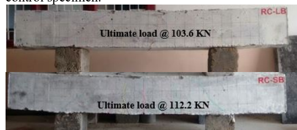
Fig 9: crack pattern of RC-SB & RC-LB
