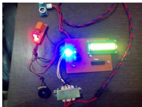
Fig.8 Ultrasonic sensor interface with Atmega 32
