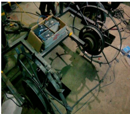
Fig.7: Two Sided seed sowing arrangement
