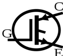
Fig 4.2: Electronic symbol for IGBT
