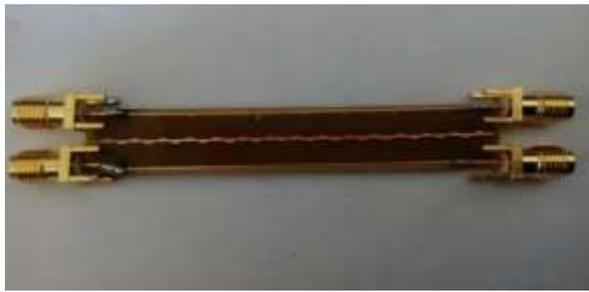
Figure 19 Double trace with continuous shield trace
