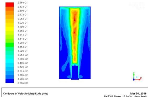
Fig 3.2 Velocity Profile outside the Metallic Foam at a given heat input 90Watts.
