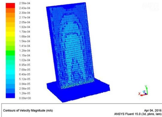
Fig 3. Velocity Profile inside Metal Foam At a given heat input 90Watts.
