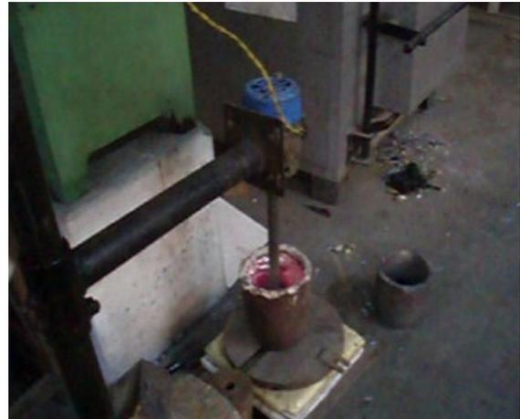
**Fig. 1 – Stirring mechanism of composite melt**
