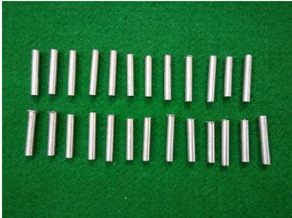
Fig. 3 –pin-on disc wear test specimens
