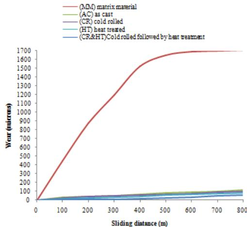
**Fig. 5 Variations of wear with the sliding distance for AA6061+4wt.% MoS<sub>2</sub> (a) MM (b) AC (c) CR (d) HT (e) CR&HT**
