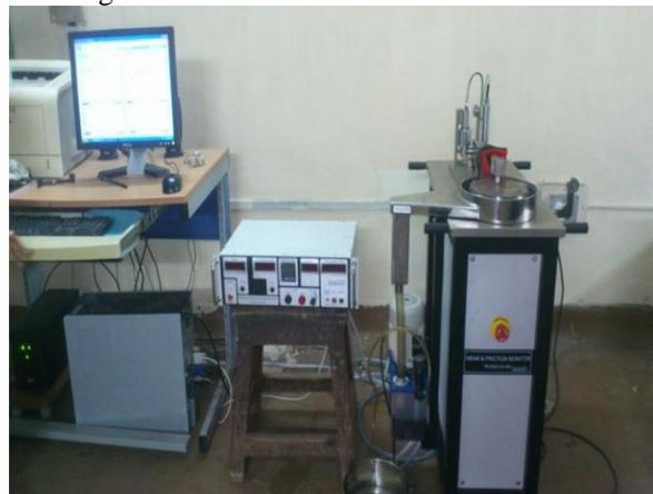
**Fig. 2 – DUCOM TR-20M-106 pin-on disc wear test apparatus**
