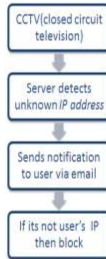
Fig.4 Flowchart for CCTV SECURITY
