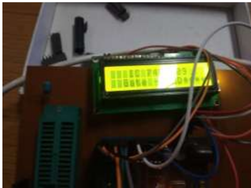
FIG5. LCD DISPLAY DISPLAYING THE OUTPUT FOR A FAULTY 7432 IC.
