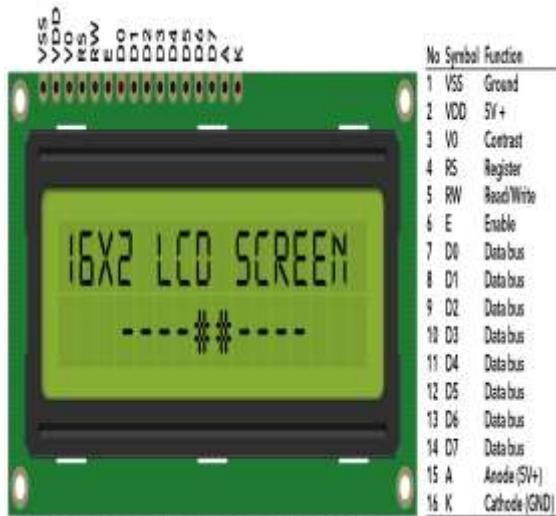
FIG3. 16*2 LCD PIN DIAGRAM
