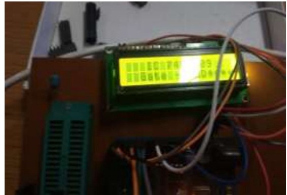
FIG6. LCD DISPLAY DISPLAYING THE GATE LEVEL OPERATION OF IC 7409
