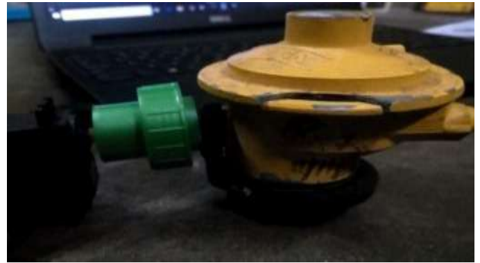
Figure 4. Servomotor coupled with Gas Valve
