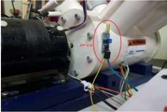
Fig9:Motor Vibration Sensor
