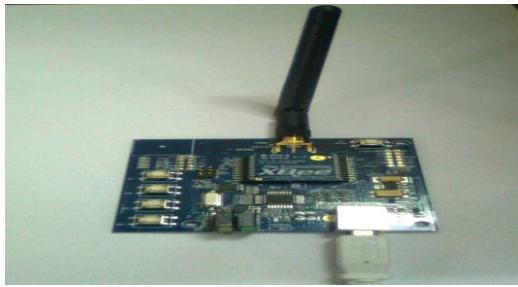
XBEE module with antenna used as transmitter.
