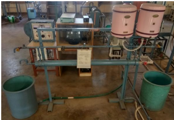
Fig. 1: Counter Current Double Pipe Heat Exchanger
